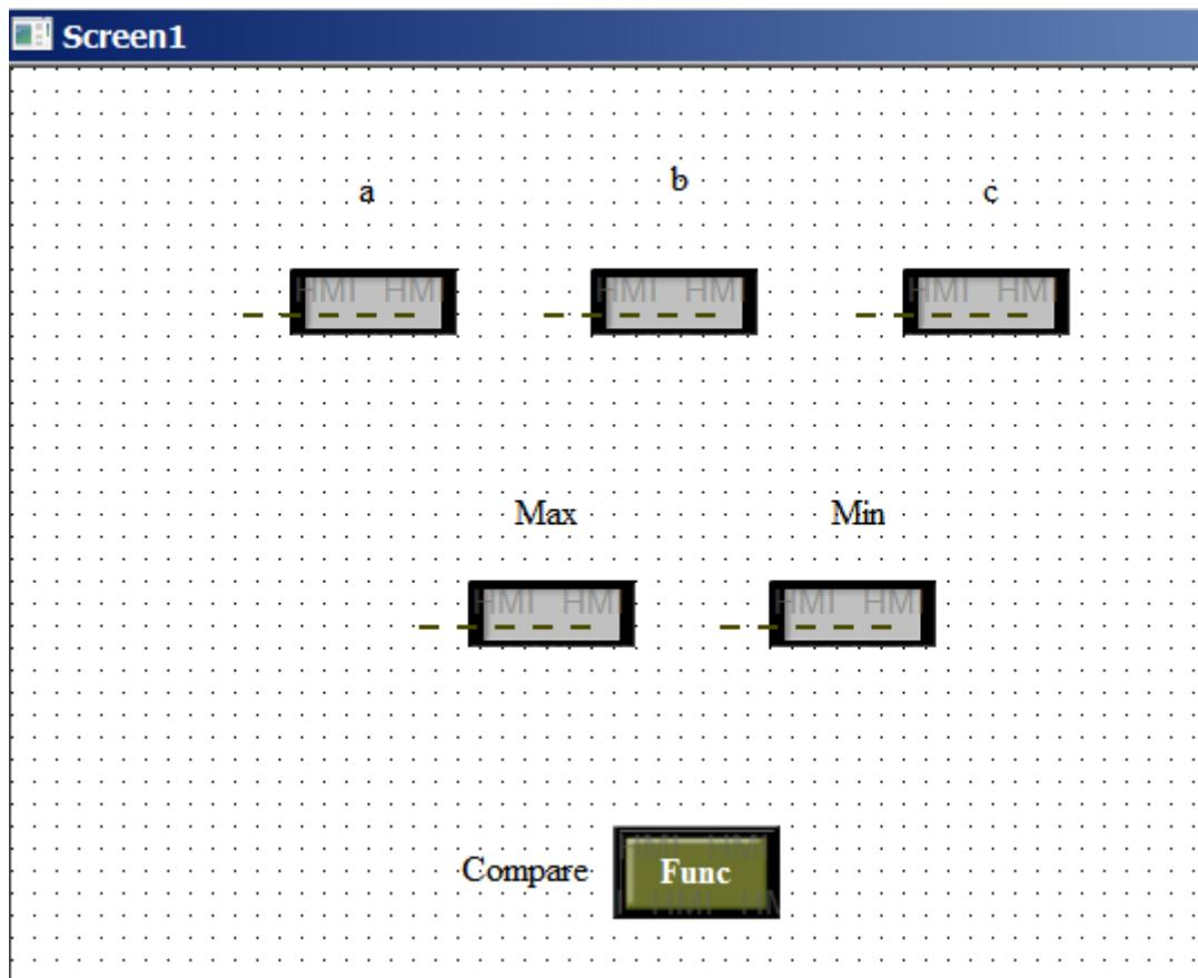
5. Download the HMI program to the TH465. Connect PLC with the TH465, power on. Input any value in a, b, c. Click Func button, the max and min value will show on the screen.
