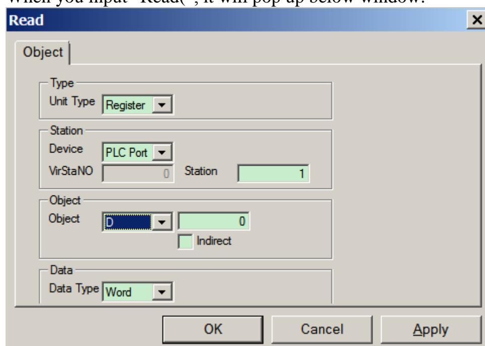
Unit type: the operation object type, select “register”
